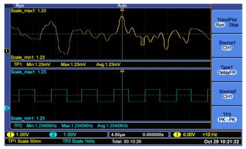
To find intermittent faults the TrendPlot <sup>™</sup> function can monitor measurements for long periods of time.
