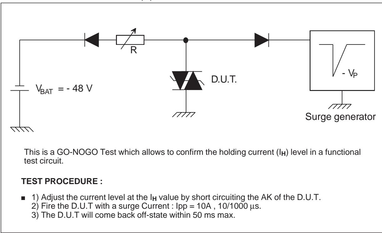
**APPLICATION CIRCUIT****Otvoltage protection and current limitation**
