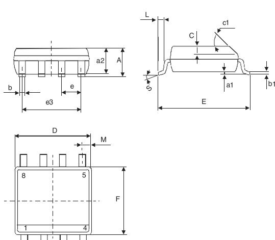
The technical drawings provide three views of the SO-8 package: a top view showing the eight pins numbered 1 through 8, a side view showing lead height (L), lead width (c1), and lead thickness (a1), and a cross-sectional view showing lead thickness (a1), lead width (c1), and lead height (L).
