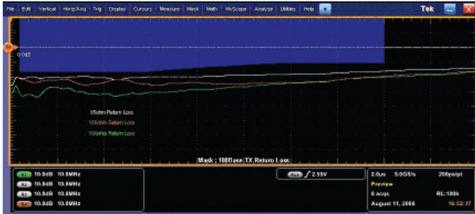
85/100/115 Ω plots for the 100BASE-TX Return Loss measurement.
