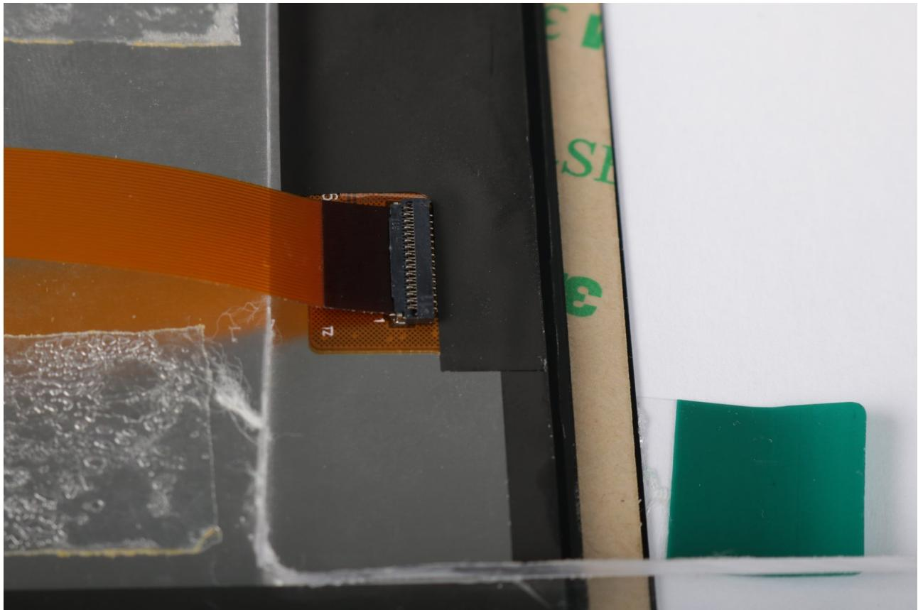
Fig. 1.5: DSI connector on the display assembly
