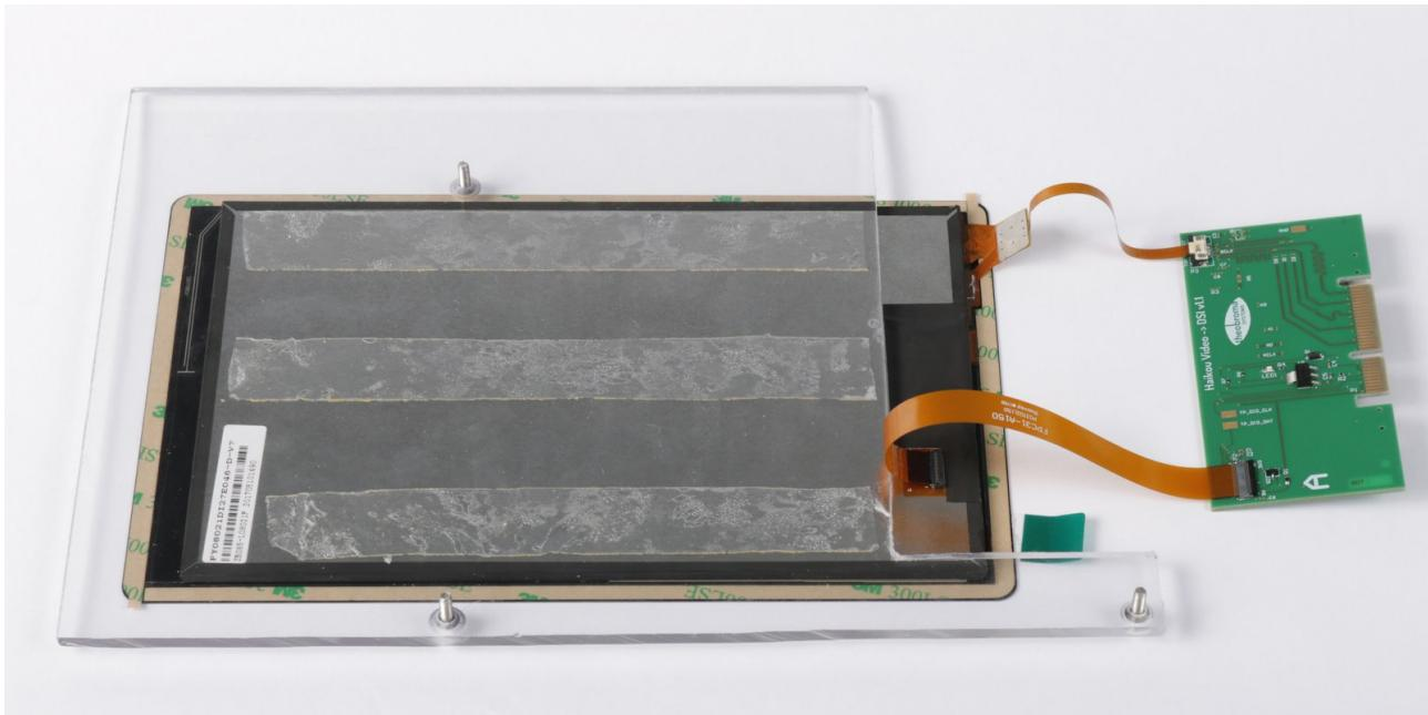
Fig. 1.2: Flat-flex cabling
