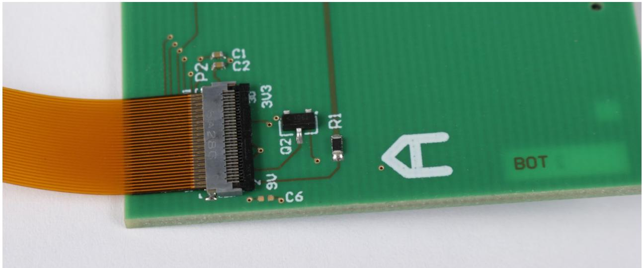
Fig. 1.4: Connector P2 (DSI) on the DSI adapter PCB
