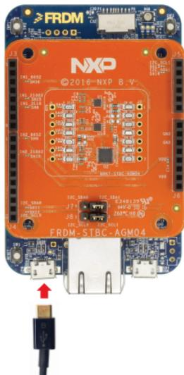
Figure 2: Connect board to computer
