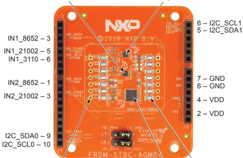
FXAS21002C 3-axis digital angular rate gyroscope
