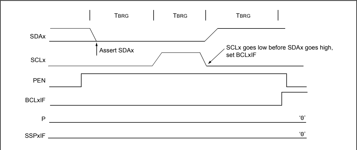
FIGURE 20-34: BUS COLLISION DURING A STOP CONDITION (CASE 2)
