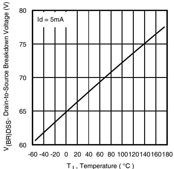
**Fig 10.** Drain-to-Source Breakdown Voltage
