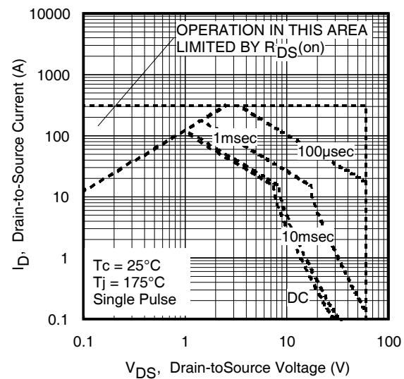
**Fig 8.** Maximum Safe Operating Area
