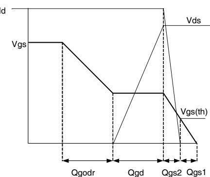
**Fig 24b.** Gate Charge Waveform
