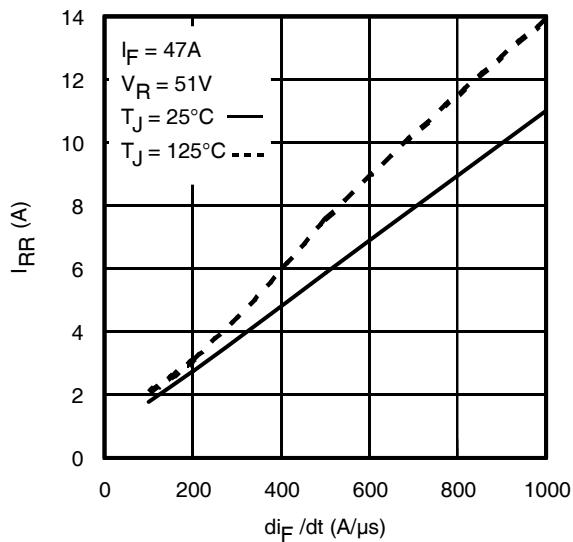
**Fig. 18** - Typical Recovery Current vs.  $di_F/dt$
