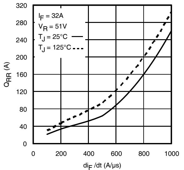
**Fig. 19** - Typical Stored Charge vs.  $di_F/dt$
