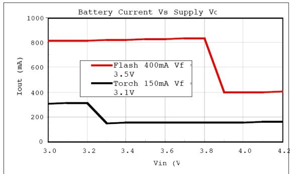
Fig. 16: Battery Current vs Supply Voltage
