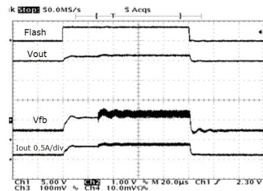
Fig. 21: Torch in 1x to Flash in 2x Mode
