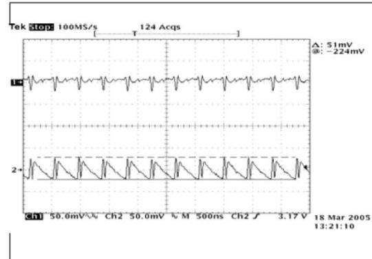
Fig. 11: Ripple 2x Torch 150mA, Ch1=V<sub>IN</sub>, Ch2=V<sub>OUT</sub>
