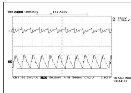
Fig. 9: Ripple 2x Flash 400mA, Ch1= $V_{IN}$ , Ch2= $V_{OUT}$
