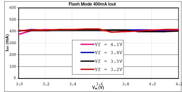
Fig. 5: Output Current vs Supply Voltage
