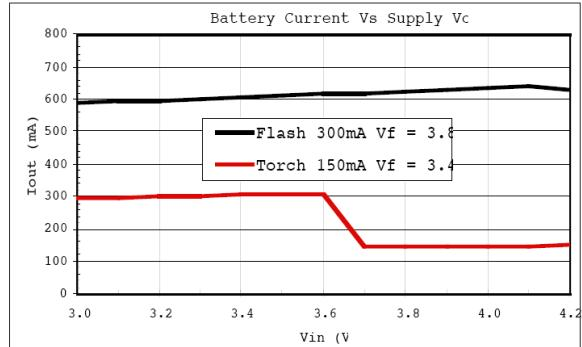
Fig. 17: Battery Current vs Supply Voltage
