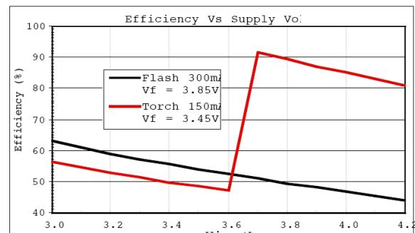
Fig. 15: Efficiency vs Supply Voltage
