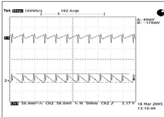
Fig. 10: Ripple 1x Torch 150mA, Ch1=V<sub>IN</sub>, Ch2=V<sub>OUT</sub>
