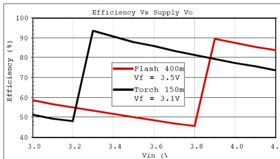
Fig. 14: Efficiency vs Supply Voltage
