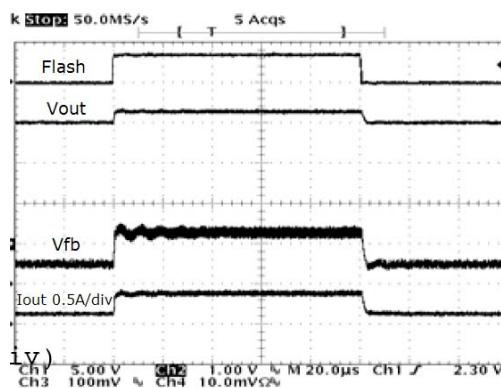
Fig. 20: Torch in 1x to Flash in 1x Mode
