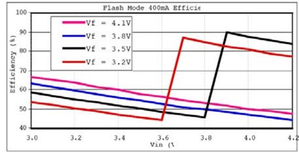
Fig. 7: Efficiency vs Supply Voltage
