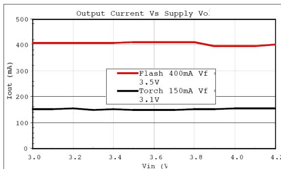
Fig. 12: Output Current vs Supply Voltage
