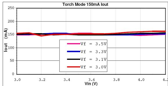
Fig. 4: Output Current vs Supply Voltage
