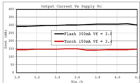
Fig. 13: Output Current vs Supply Voltage
