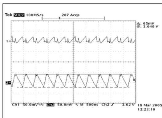
Fig. 8: Ripple 1x Flash 400mA, Ch1= $V_{IN}$ , Ch2= $V_{OUT}$
