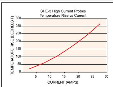
IDL current ratings are defined as the maximum current at which the temperature rise of the probe does not exceed 144°F (80°C) for a single probe in free air at ambient temperature for one hour.
