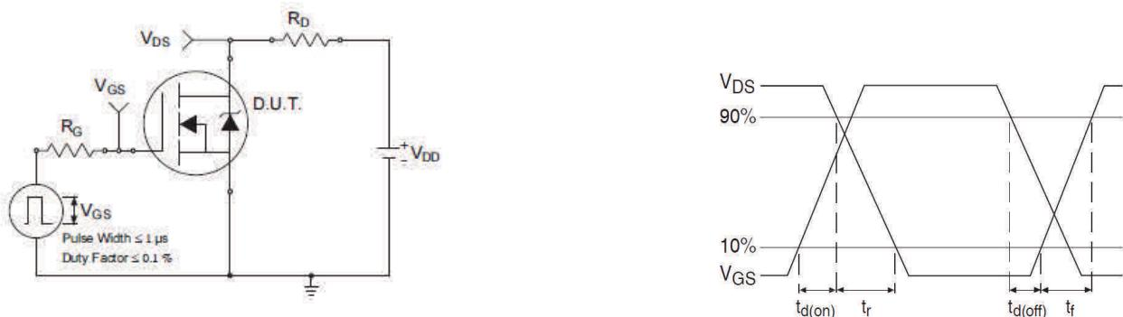
**Fig 18a.** Switching Time Test Circuit
