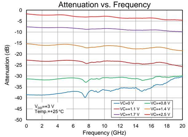
Measured Positive Attenuation Slope Performance
