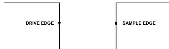
Figure 65. SPI Mode 3, SCLK Edges
