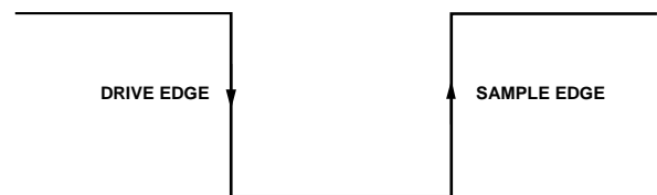
Figure 65. SPI Mode 3, SCLK Edges
