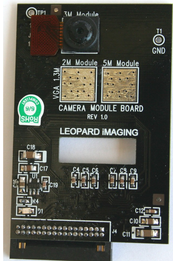
Figure 10. 3M Camera Board
