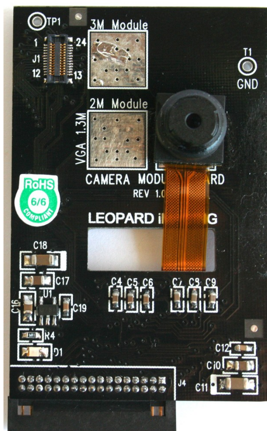
Figure 11. 5M Camera Board
