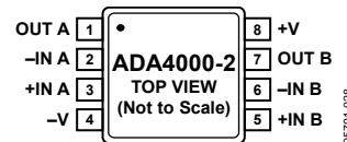
Figure 4. 8-Lead MSOP (RM-8)
