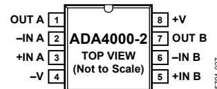
Figure 3. 8-Lead SOIC (R-8)
