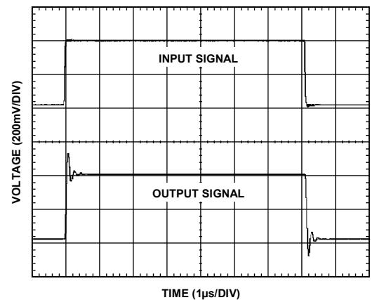
Figure 31. Capacitive Load Drive Without Snubber Network
