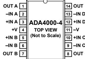
Figure 5. 14-Lead SOIC (R-14)
