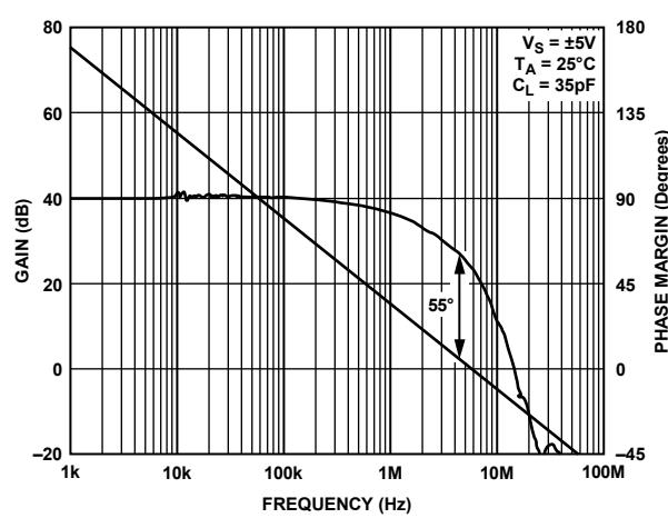
Figure 12. Open-Loop Gain and Phase Margin vs. Temperature,  $V_S = \pm 5\text{ V}$
