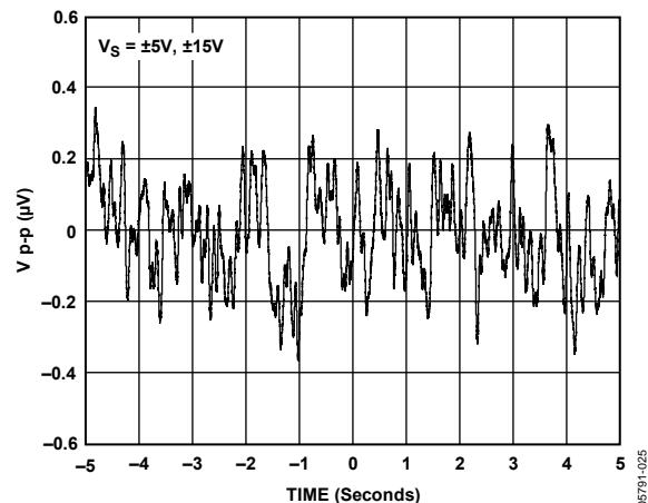
Figure 28. 0.1 Hz to 10 Hz Input Voltage Noise
