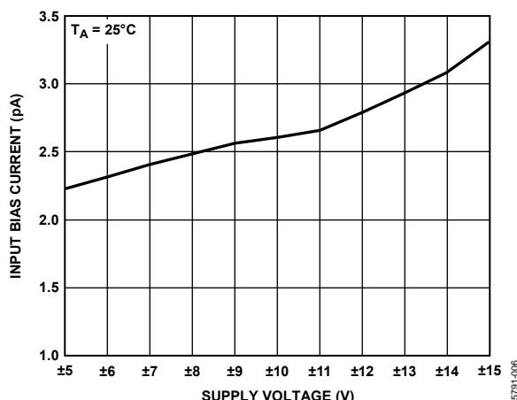
Figure 19. Input Bias Current vs. Supply Voltage
