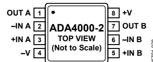
Figure 4. 8-Lead MSOP (RM-8)
