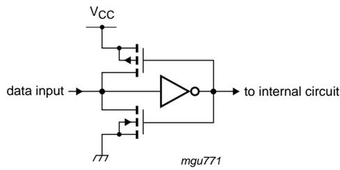
**Fig 4. Bus hold circuit**
