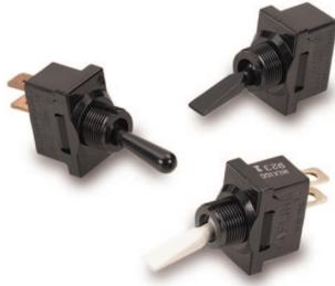
The D-Series single pole compact high current toggle switches are ideal for applications with back panel size constraints. These switches feature self-cleaning contacts and ratings up to 20A 125VAC, 10A 250VAC, 1 1/2 HP 125-250VAC. With an economical double insulated all-nylon construction, these switches figure prominently in the Environmental Controls, Marine, Food Service, Vacuum Cleaner and various other general purpose markets with stringent current carrying requirements.
