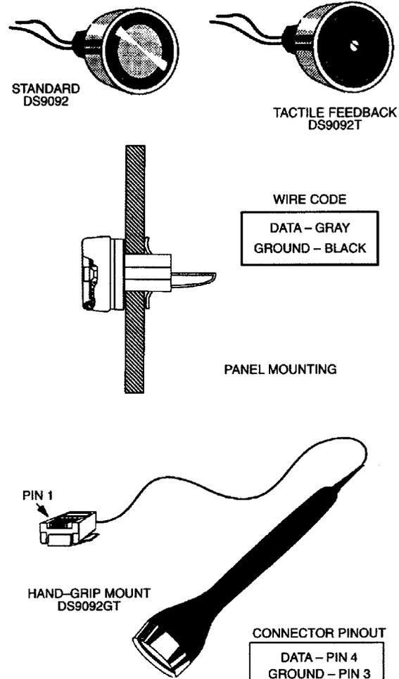
environments. This type of probe is best suited for designs where the iButton is brought into contact with the reader.
