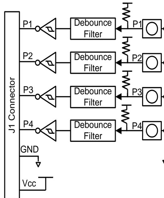
Figure 1. BTN circuit diagram.
