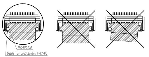
♦ Checking the Locking Condition
