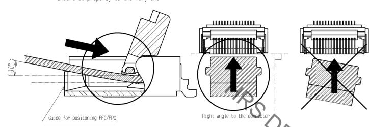
2. Do not insert the FFC/FPC diagonally from above.
