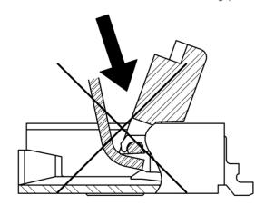
3. Do not rotate the actuator when FFC/FPC TAB is on right and left guides for positioning FFC/FPC. Make sure the position of FFC TAB and guides before rotate the actuator.
