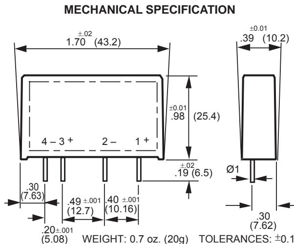
Figure 1 – DS relays; dimensions in inches (mm)
