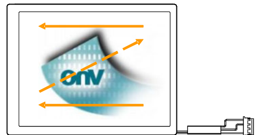
Fig. 2 Reverse scan (Pin4, DPS = High)
