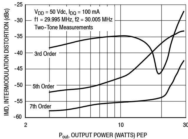
**Figure 19. Intermodulation Distortion Products versus Output Power — 30 MHz**
