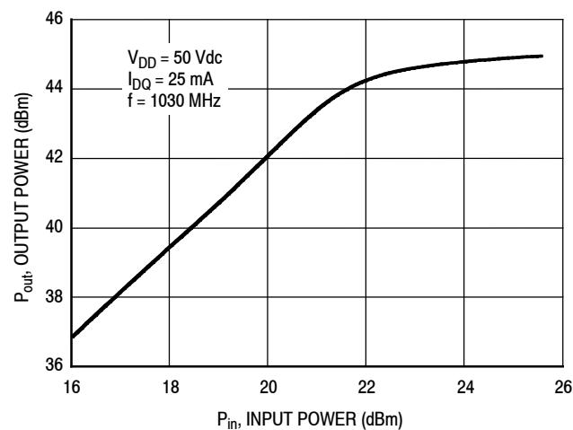
**Figure 35. CW Output Power versus Input Power**
