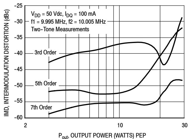
**Figure 18. Intermodulation Distortion Products versus Output Power — 10 MHz**
