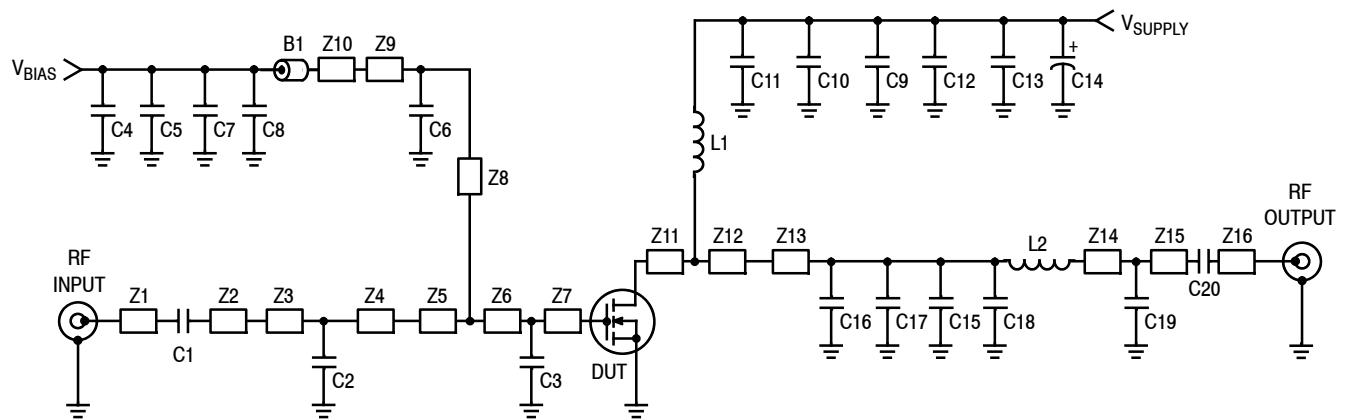
**Figure 33. MRFE6VS25NR1 Narrowband Reference Circuit Schematic — 1030 MHz**
