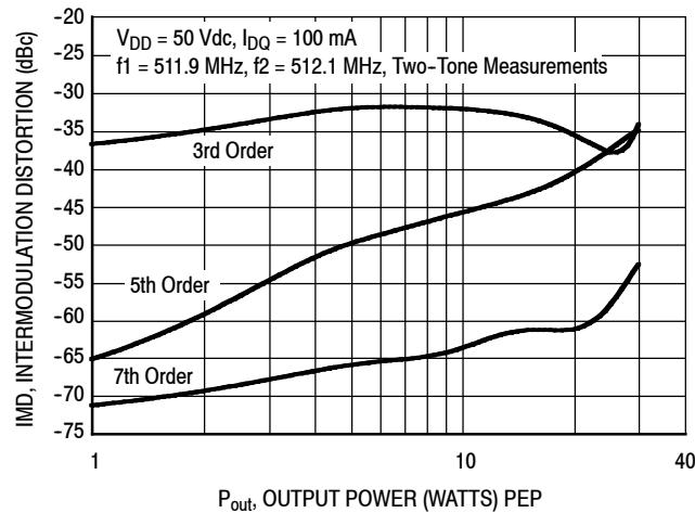
**Figure 30. Intermodulation Distortion Products versus Output Power — 512 MHz**
