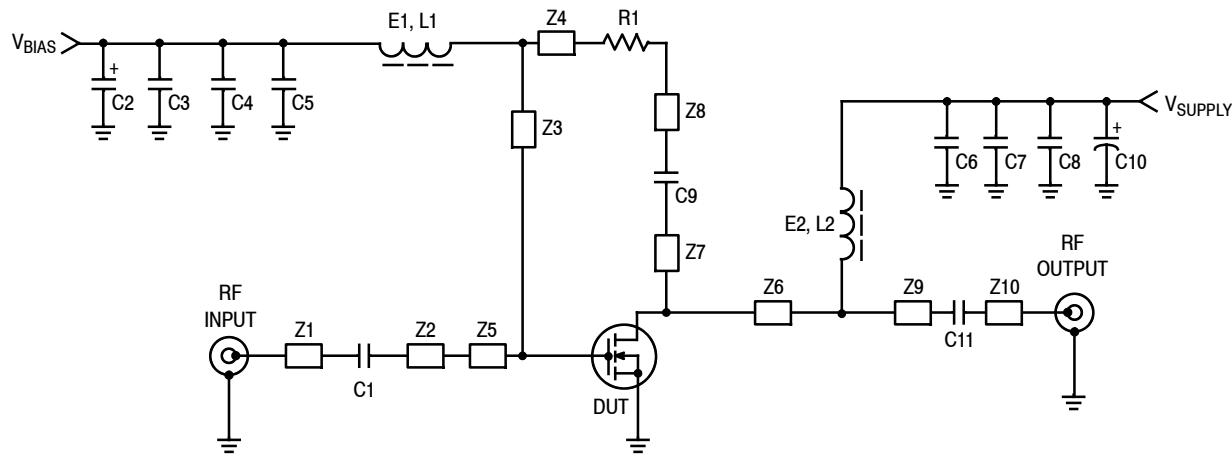
**Figure 12. MRFE6VS25NR1 Broadband Reference Circuit Schematic — 1.8-30 MHz**
