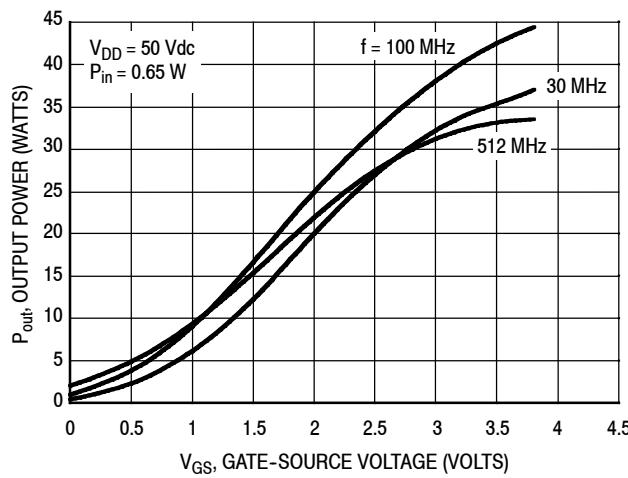
**Figure 24. CW Output Power versus Gate-Source Voltage at a Constant Input Power — 0.65 W**
