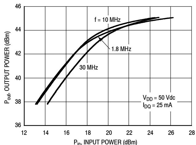
**Figure 15. CW Output Power versus Input Power**
