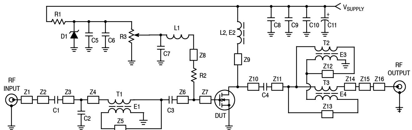
**Figure 22. MRFE6VS25NR1 Broadband Reference Circuit Schematic — 30-512 MHz**
