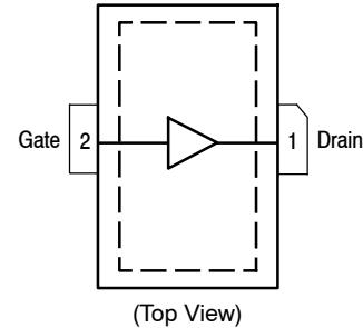
Note: The backside of the package is the source terminal for the transistor.
