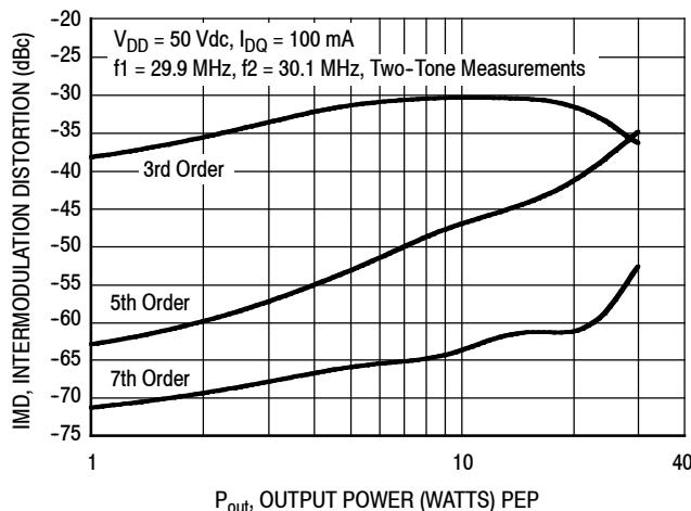
**Figure 28. Intermodulation Distortion Products versus Output Power — 30 MHz**
