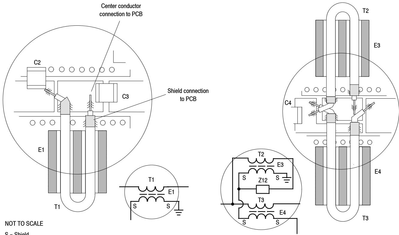
**Figure 21a. Detailed View of Semi-flex Cables with Shields and #61 Multi-aperture Cores**
