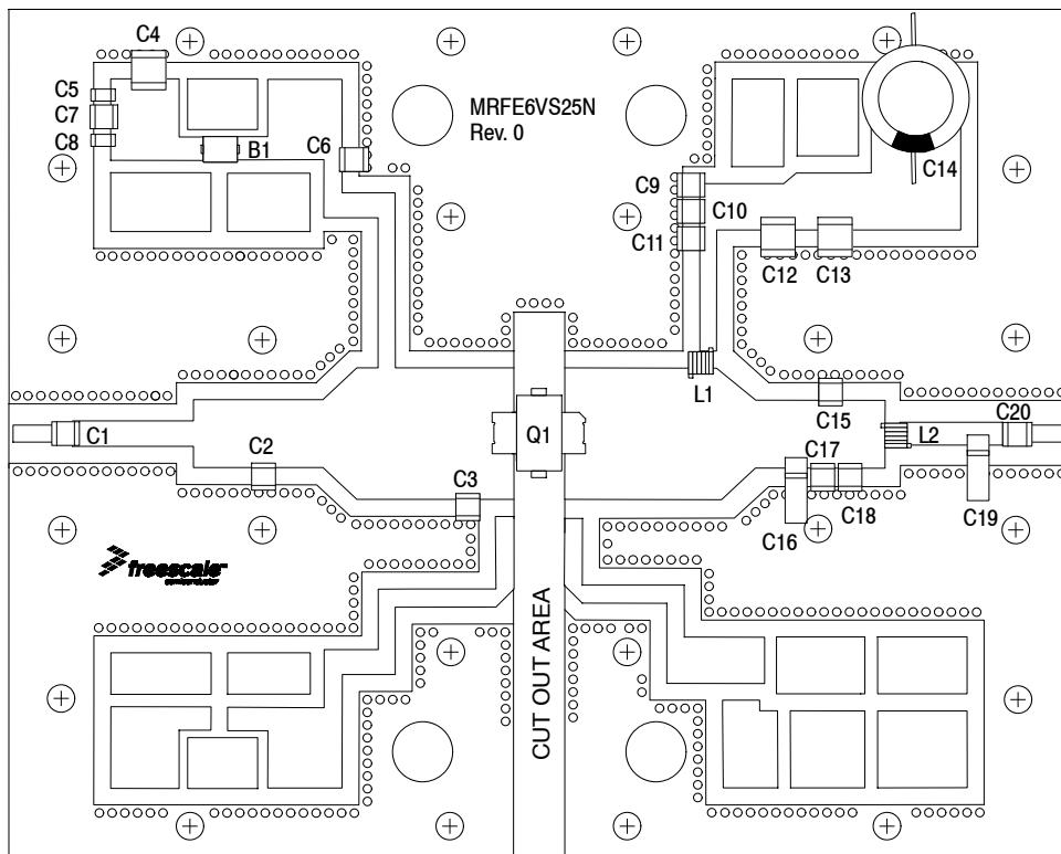
**Figure 32. MRFE6VS25NR1 Narrowband Reference Circuit Component Layout — 1030 MHz**
