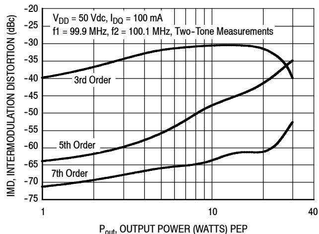
**Figure 29. Intermodulation Distortion Products versus Output Power — 100 MHz**
