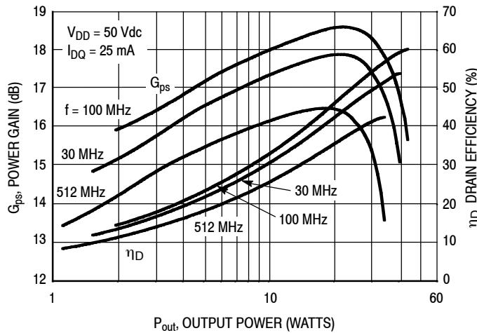
**Figure 27. Power Gain and Drain Efficiency
