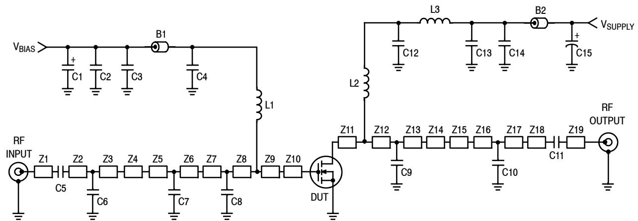
**Figure 6. MRFE6VS25NR1 Narrowband Test Circuit Schematic — 512 MHz**
