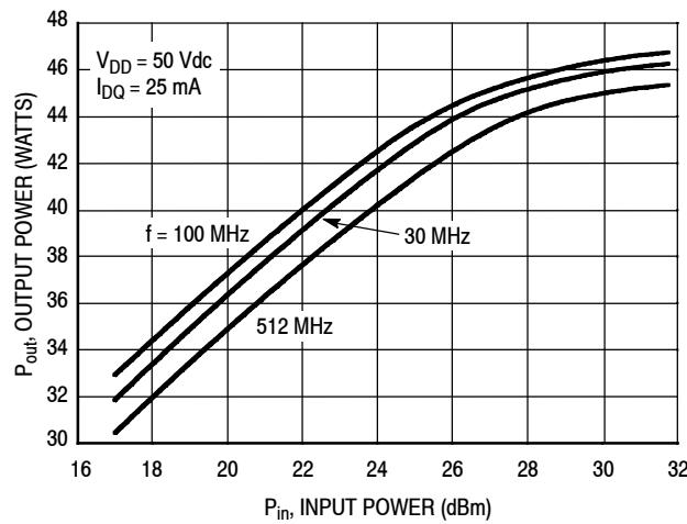
**Figure 26. CW Output Power versus Input Power**
