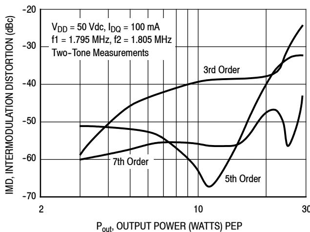
**Figure 17. Intermodulation Distortion Products versus Output Power — 1.8 MHz**
