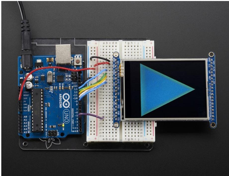
If you're having difficulties, check the serial console. The first thing the sketch does is read the driver code from the TFT. It should be `0x9341` (for the `ILI9341` controller inside)
