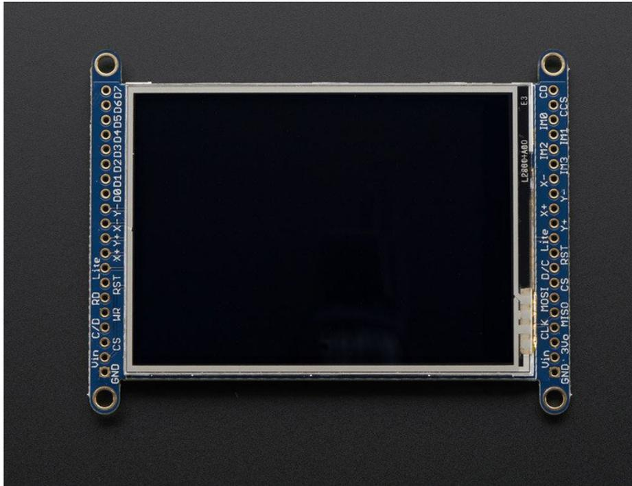
We tried to make this TFT breakout useful for both high-pin microcontrollers that can handle 8-bit data transfer modes as well as low-pincount micros like the Arduino UNO and Leonardo that are OK with SPI.
