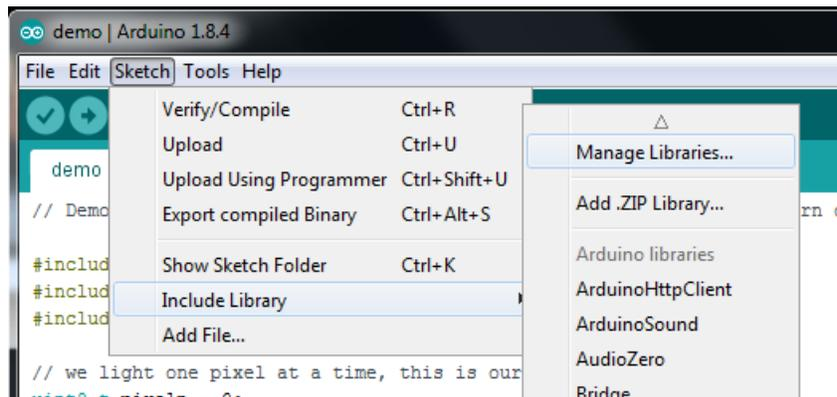
Search for the **Adafruit\_GFX** library and install it. If using an older Arduino IDE (pre-1.8.10), also locate and install **Adafruit\_BusIO**.
