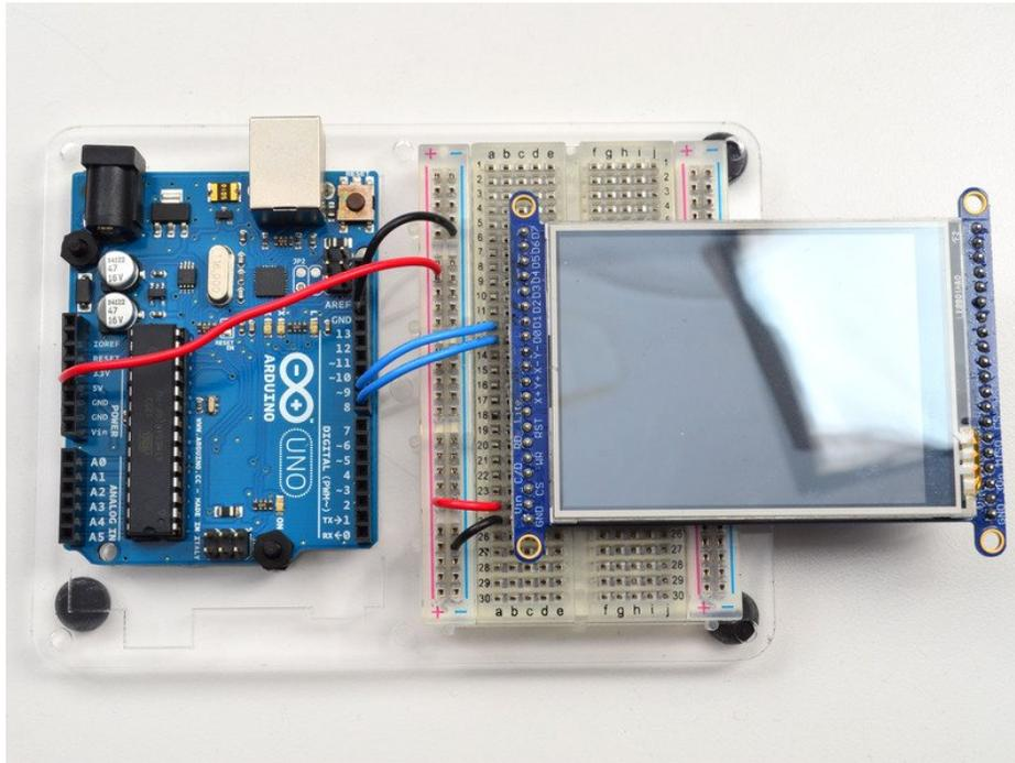
Begin by connecting **D0** and **D1** to digital **#8** and **9** respectively as seen above. If you're using a Mega, connect the TFT Data Pins **D0-D1** to Mega pins **#22-23**, in that order. Those Mega pins are on the 'double' header.
