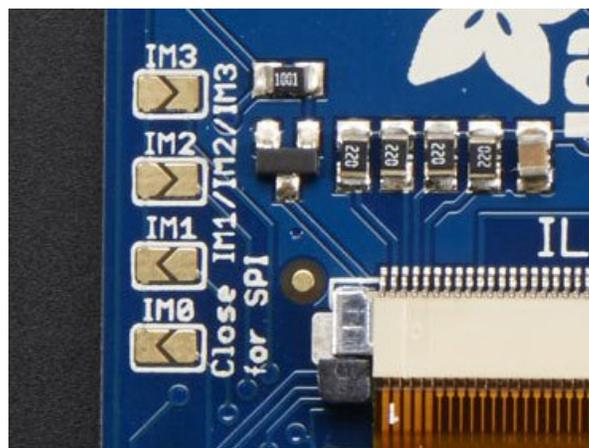
With your soldering iron, melt solder to close the three jumpers indicated **IM1** **IM2** and **IM3** (do not solder closed **IM0**!)
