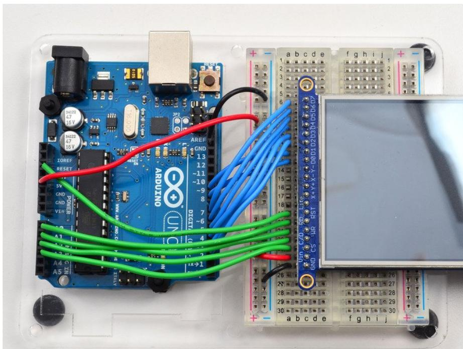
You can connect the seventh pin **RST** (Reset) to the Arduino Reset line if you'd like. This will reset the panel when the Arduino is Reset. You can also use a digital pin for the LCD reset if you want to manually reset. There's auto-reset
