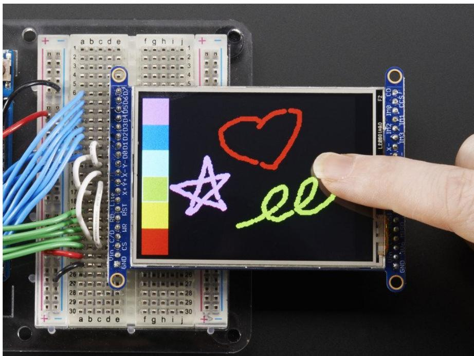
This display has a controller built into it with RAM buffering, so that almost no work is done by the microcontroller. **The display can be used in two modes: 8-bit or SPI.** For 8-bit mode, you'll need 8 digital data lines and 4 or 5 digital control lines to read and write to the display (12 lines total). SPI mode requires only 5 pins total (SPI data in, data out, clock, select, and d/c) but is slower than 8-bit mode.
