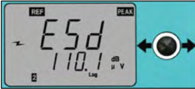
Figure 7. Modifying the ESD event threshold
