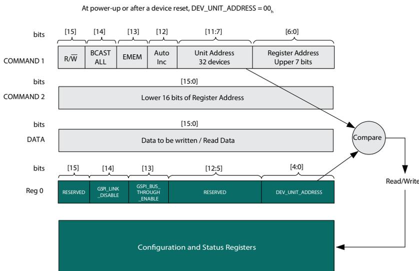
**Figure 3-24: Internal Register Map Functional Block Diagram**
