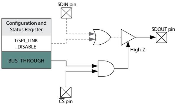
**Figure 3-15: GSPI\_BUS\_THROUGH\_ENABLE Operation**
