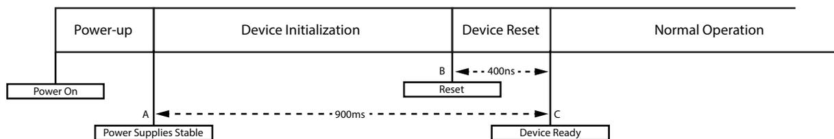
**Figure 3-3: Device Power Up and Reset Sequencing**
