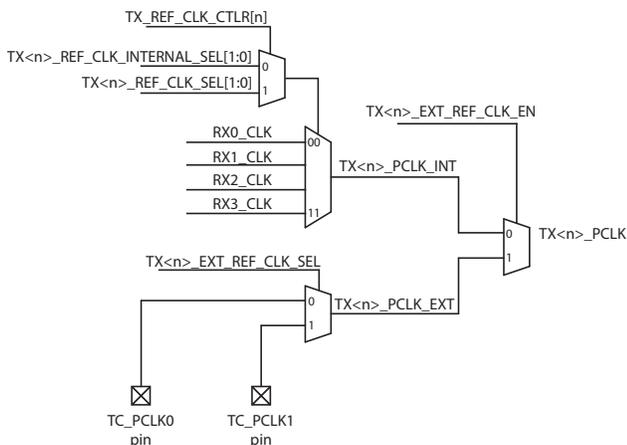
Figure 3-6: Tx PLL Input Clock Selection Block
