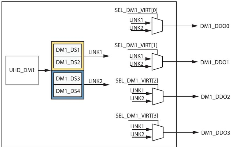
**Figure 3-13: Output Link Assignment Selection**
