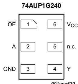
Fig. 5. Pin configuration SOT886 (XSON6)
