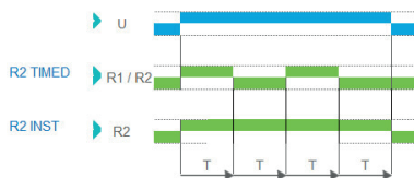
Function Ht - Interval summation time relay
