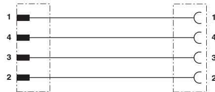
Contact assignment of M8 plugs/sockets
