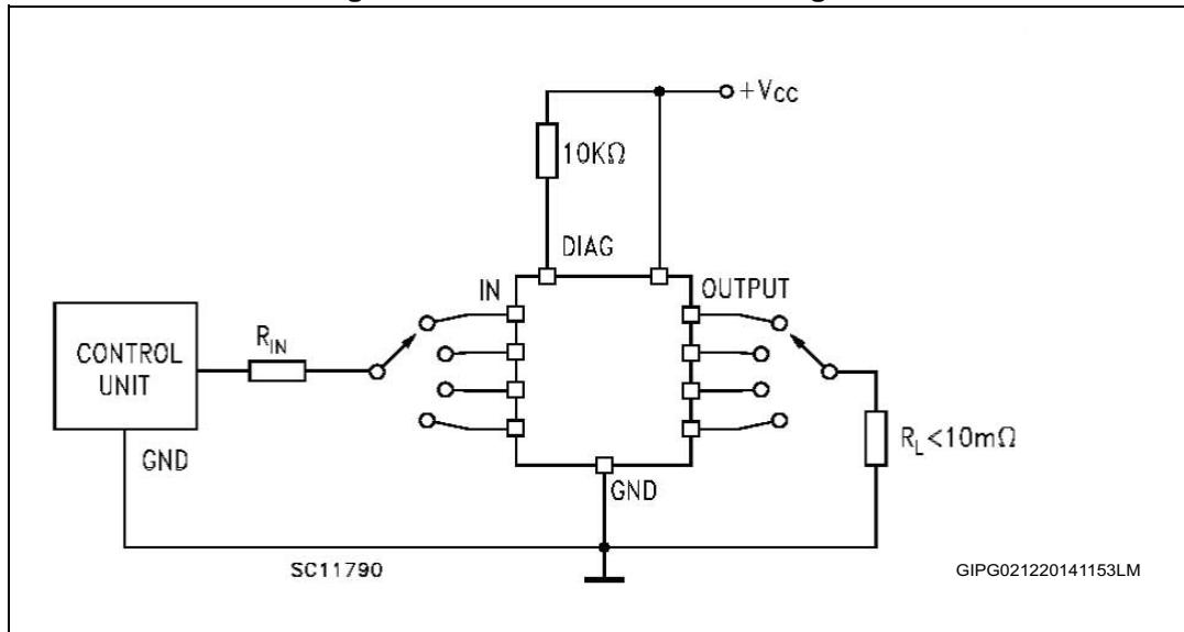
**Figure 6.  $I_{LGND}$  test configuration**
