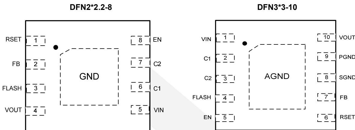
**Figure 1 Pin Assignment (Top View)**
