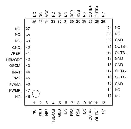
Note: Please connect the corner pad and the exposed pad to the PCB ground pattern when using the QFN package.
