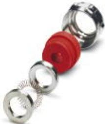
EMC half screw connection Pg21, for metal housings of sizes 2-4, consisting of rubber seal, iris spring, cone disks and pressure screw, for size 1 housings, cable shielding range [mm] 7.5-12, cable [mm] 9-13
