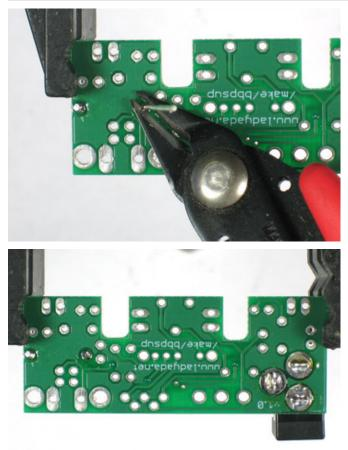
Now use yoru diagonal cutters to clip the long leads just above the solder joint.
