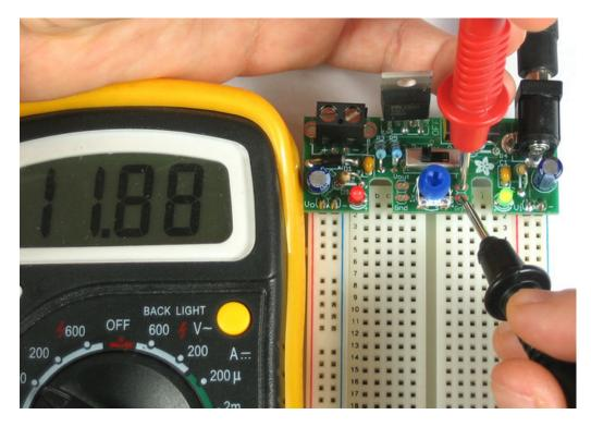
For example, this photo is me testing the output of the right hand side with a 12VDC regulated power adapter attached. The voltage is within 200mV of 12V. The green LED indicates that there is power on the right hand side.
