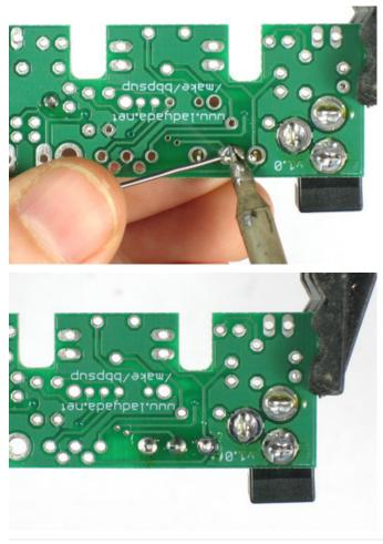
Tape or hold the switch in place while you solder all three pins.
