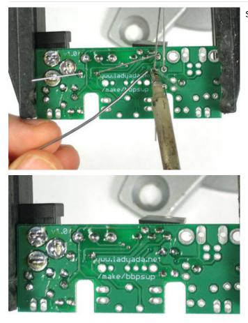
Solder and clip the three resistors.
