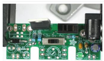
Now we need a way to select which resistor is connected to the regulator. For that we use a 3-way switch. The switch can only go in one way.
