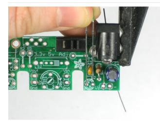
We will finish up the 'high voltage' power supply side by placing the green indicator LED. This LED will let us know that power is working! LEDs are diodes so they are polarized. If not placed correctly they will not work! So make sure you get this right.
