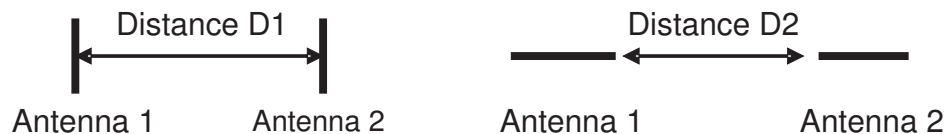
Figure D-1. Distance Between Antennas (Top View)
