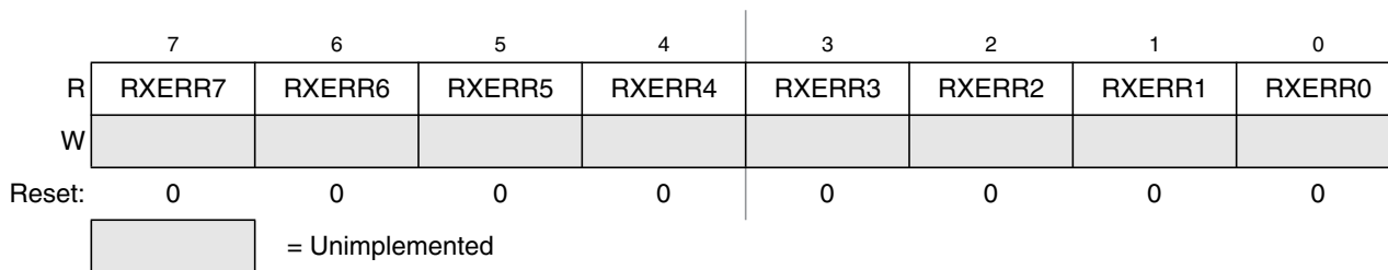
Figure 10-17. MSCAN Receive Error Counter (CANRXERR)
