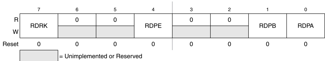
Figure 4-15. Reduced Drive Register (RDRIV)
