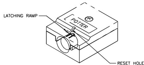
To unlatch the HUB-M, insert a small pointed object, such as a pocket screwdriver or paper clip into the reset hole. The unit unlatches when the cap is released.
