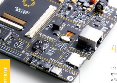
Figure 10: MicroSD card slot view
