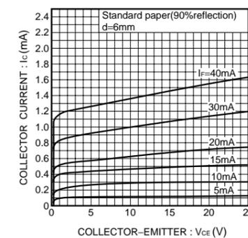
Fig.8 Output characteristics
