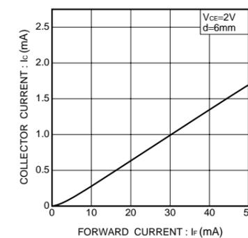
Fig.7 Collector current vs. forward current
