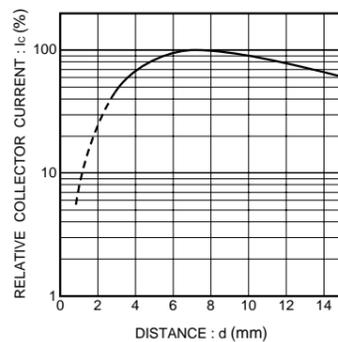
Fig.1 Relative output vs. distance
