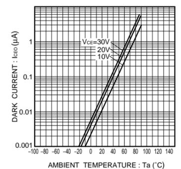
Fig.9 Dark current vs. ambient temperature
