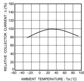
Fig.6 Relative output vs. ambient temperature
