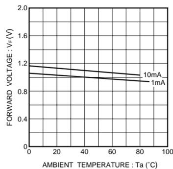
Fig.4 Forward voltage vs. ambient temperature
