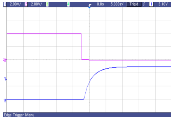
Fig. 68 AVO75-48S05 typical start-up from CNT on
