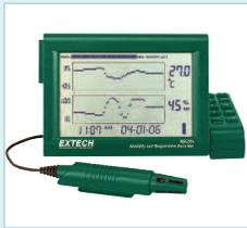
Desk mount configuration with easy to program swivel arm control panel plus probe with remote cable for reaching into ducts and humidity chambers
