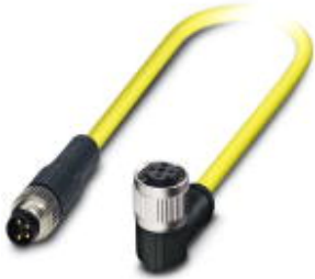
Sensor/Actuator cable, 4-position, PVC, Yellow RAL 1021, Plug straight M8, on Socket angled M12-SPEEDCON, A-coded, Cable length: 1.5 m
