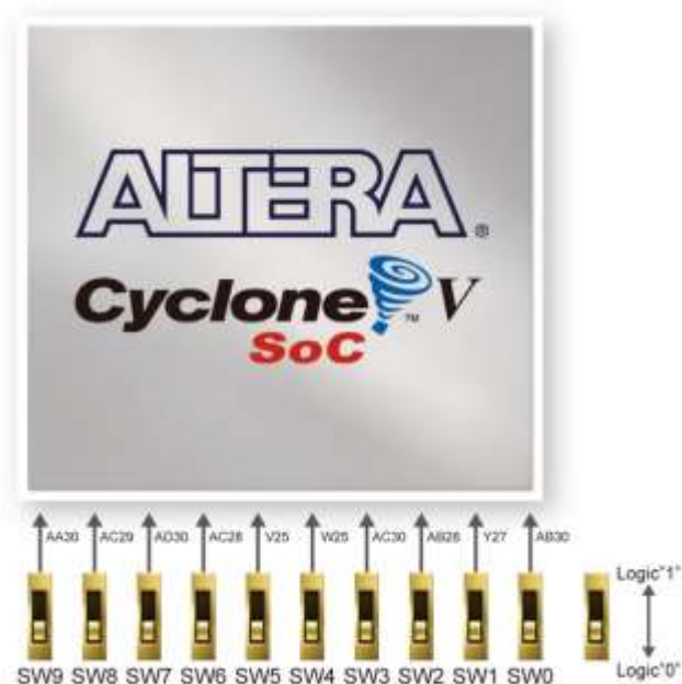
Figure 3-16 Connections between the slide switches and the Cyclone V SoC FPGA
