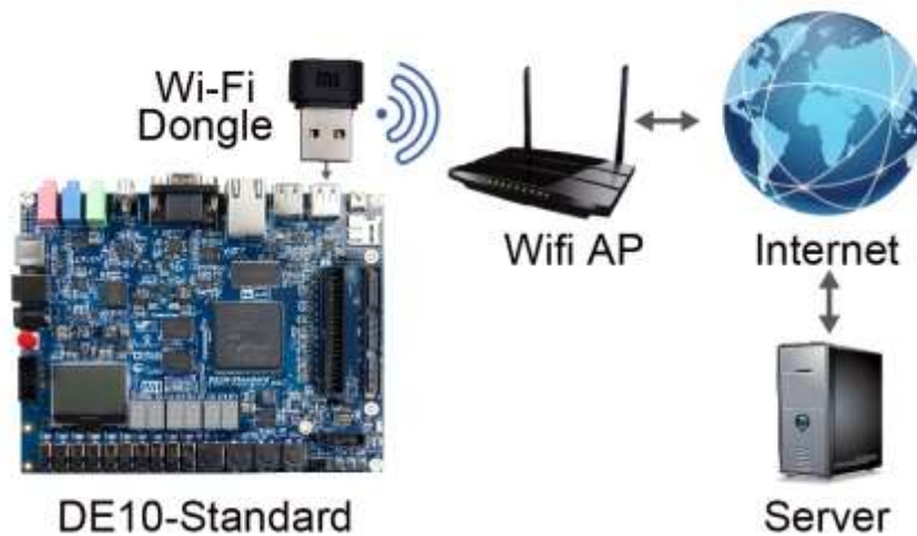
Figure 6-15 System diagram of USB Wi-Fi dongle
