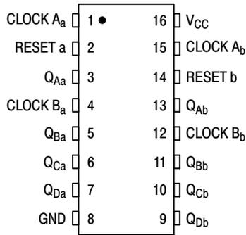
Figure 1. Pin Assignment
