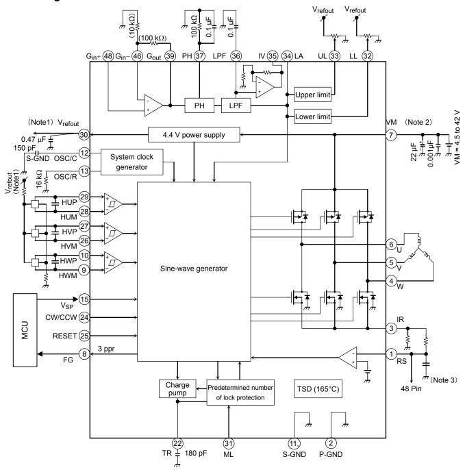
Note 1: An oscillation prevention capacitor should be connected to the  $V_{refout}$  pin at a location as close to the TB6585AFTG as possible.
