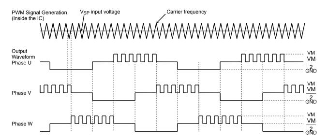
Note: The above U-phase waveform shows the behavior of the U-phase output signal when a resistor is connected between the U and VM pins and also between the U pin and ground to obtain  $\frac{VM}{2}$ . Likewise, resistors are connected to the V and W pins.  $\frac{VM}{2}$  indicates the high-impedance state.
