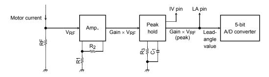
\*: Gain =  $(R_1 + R_2)/R_1$ ,  $R_3 = 100 k\Omega$ ,  $C_1 = 0.1 \mu F$
