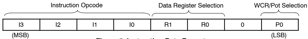
Figure 5. Instruction Byte Format
