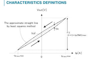
$\cdot$  When Ip\_{(RMS)}max is bigger than the value of If, Ip\_{(RMS)}max restricts it to the value of If.
